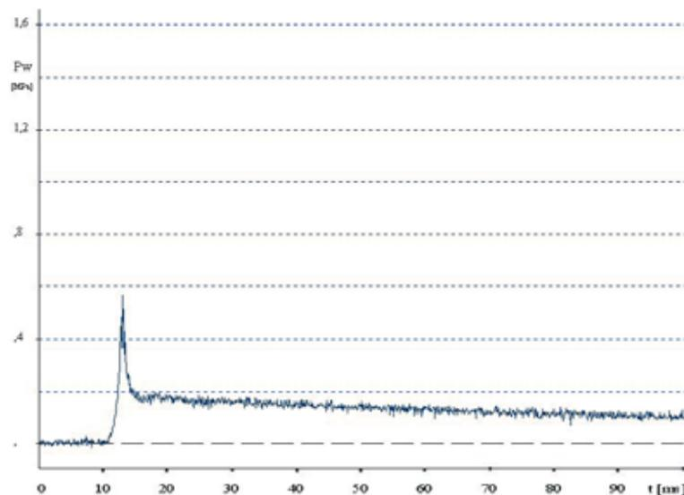
Fig. 8. Exemplary graph of one work cycle of the two-cycle miniature shaftless engine with the free piston
