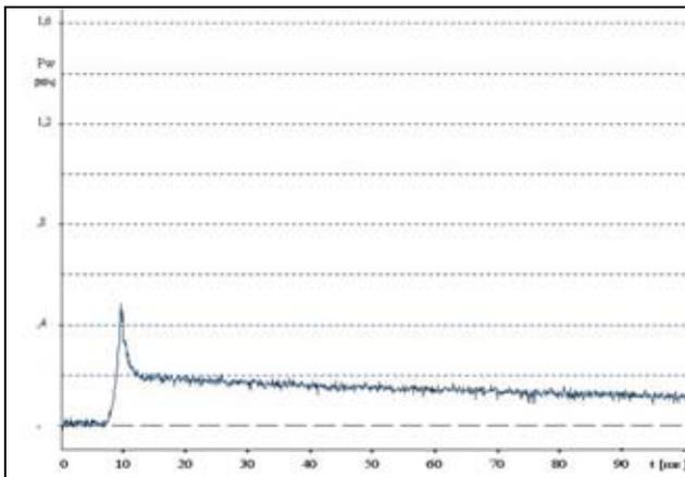
Fig. 6. Exemplary graph of air compression pressure in the combustion chamber of a two-cycle miniature shaftless engine with free piston and minimal tension of the regulating spring
