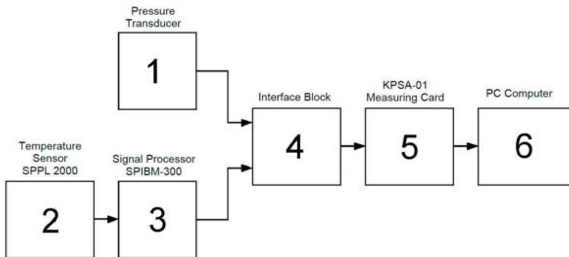
Fig. 5. The block schema of measuring system with the computer data acquisition and recording
