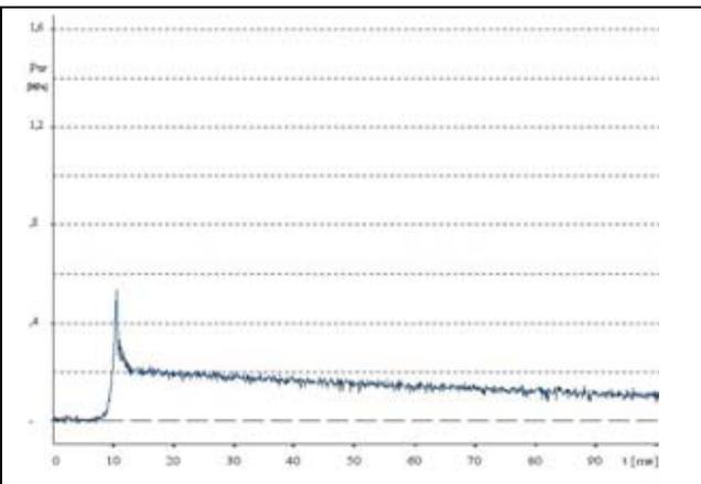
Fig. 7. Exemplary graph of compressed air pressure heated up by glow plug (catalytic igniter) in the combustion chamber of a two-cycle miniature shaftless engine with free piston
